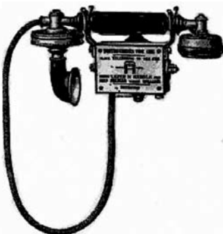
A typical early all metal "traction" phone for tramways and collieries, the Model K71
